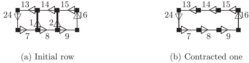
Fig. 7. Contraction of the first row represented in the dual combinatorial map (Fig. 3(b)). The edges to be removed are represented by thick lines.
